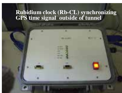
Figure-3: Time recording device that used the Rubidium clock and operation method in tunnel
