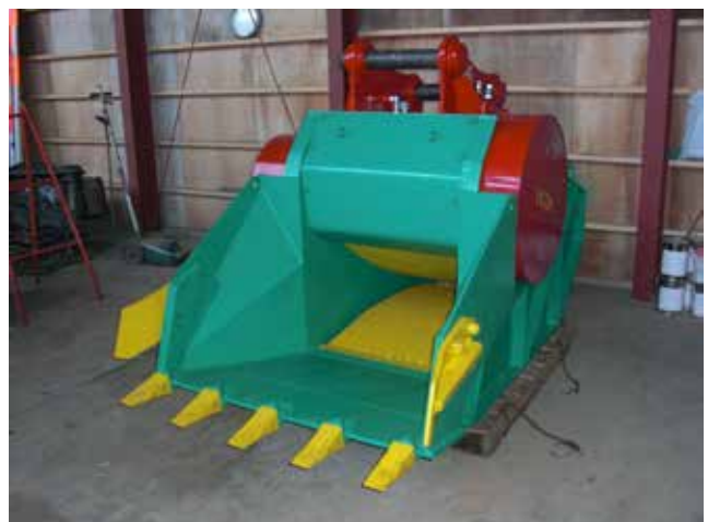
Picture 1, Bucket Crusher (FU-70)
